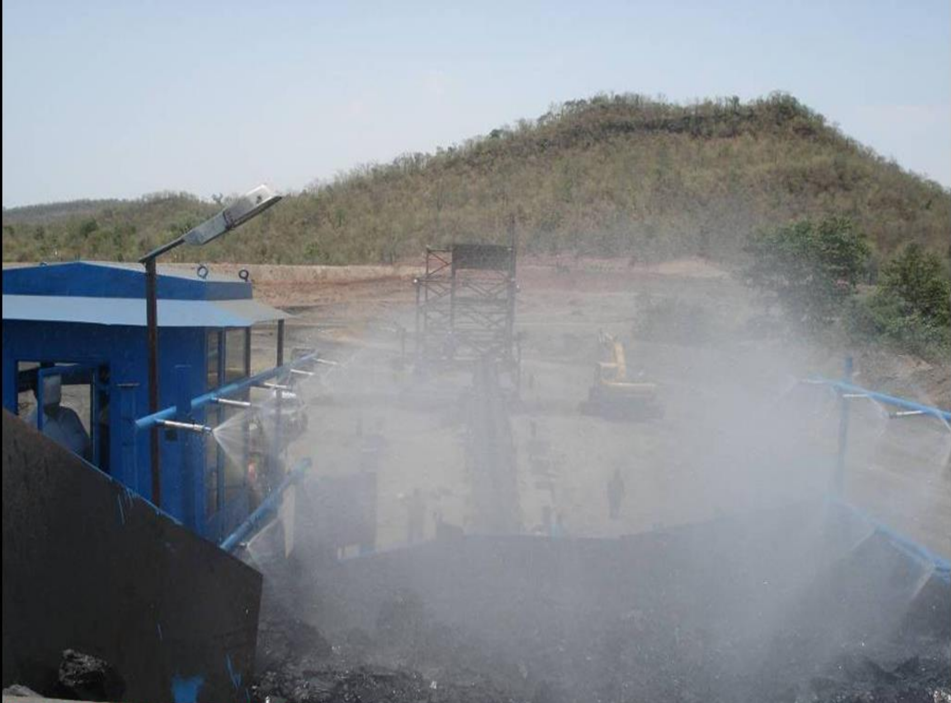
Water Spraying Arrangements at Feeder Breaker of BPA OC II Extn. BPA Area
