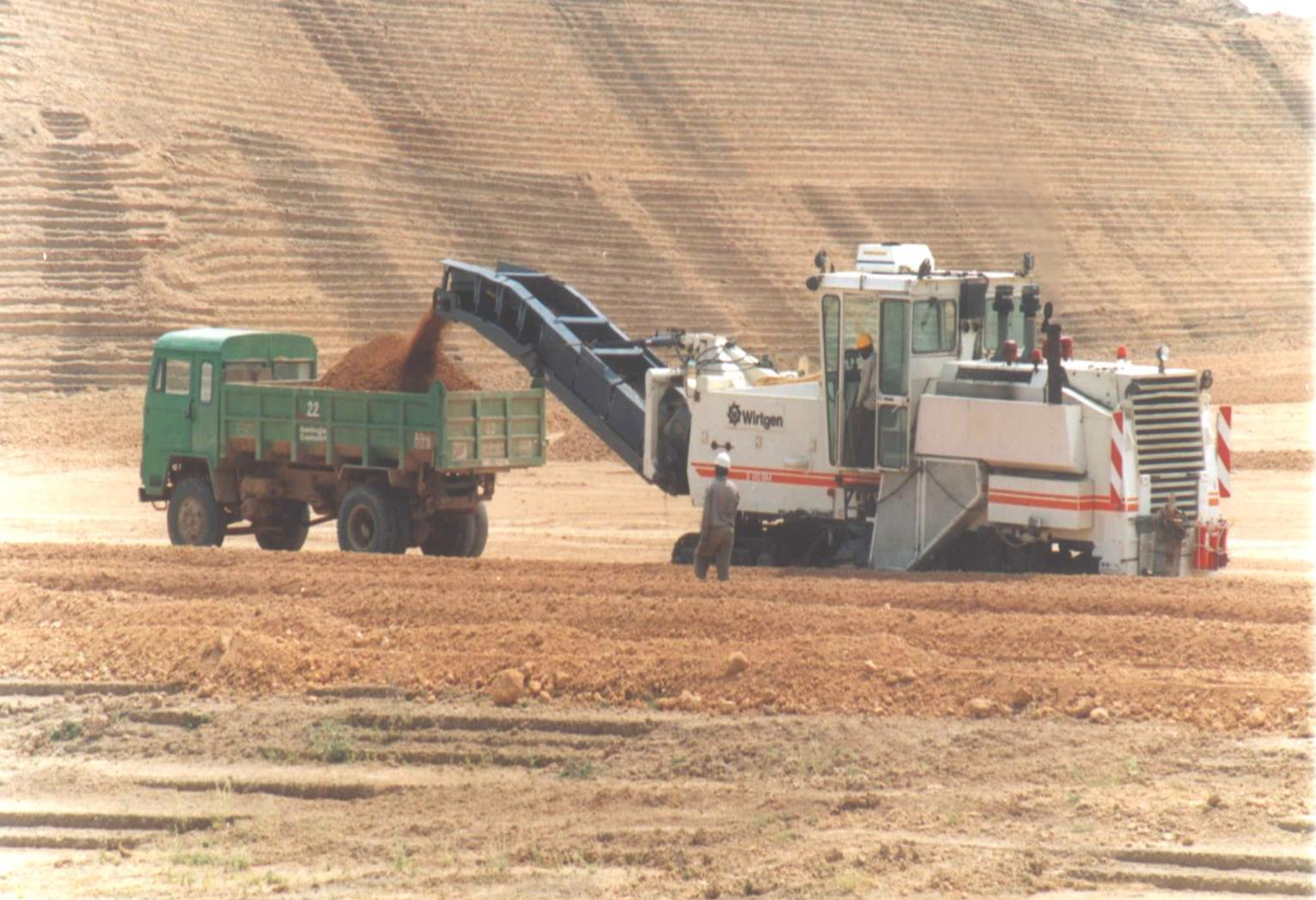
Direct Tipper Loading By Surface Miner
