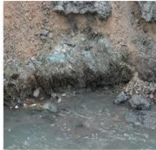
Copper sulphate stained sediment and rock - drainage trench below the Slag Dump, Nkana Mine, Kitwe
