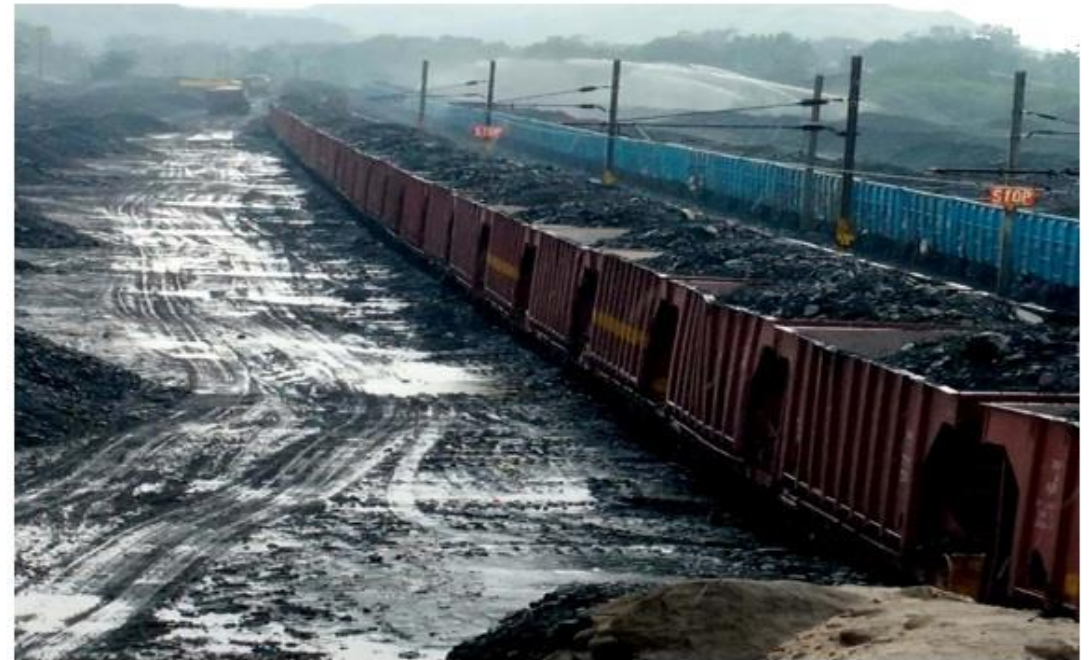
Pic. 04: Ghugus Railway siding of WCL with fixed sprinklers
