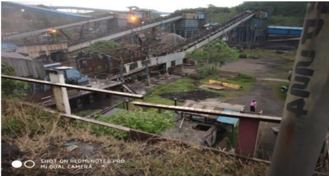
Pic. 01: Un-covered conveyor belt at CHP in Lingraj Mine of MCL
